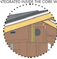
HVAC DUCTWORK AND LIGHTING INTEGRATED INSIDE THE CORE WALL
