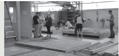
In addition to designing the house, KSU architecture students constructed wall and roof panels in their fabrication shop
